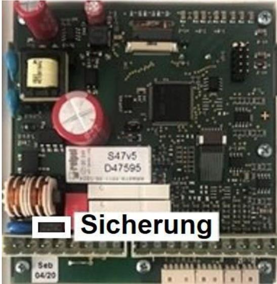
If the controller has no function and display despite the mains voltage being switched on, the internal device fuse may be defective.
